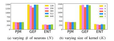
Fig. 6: RMSE of PhaCIA-TCNs on validation sets of three datasets.
